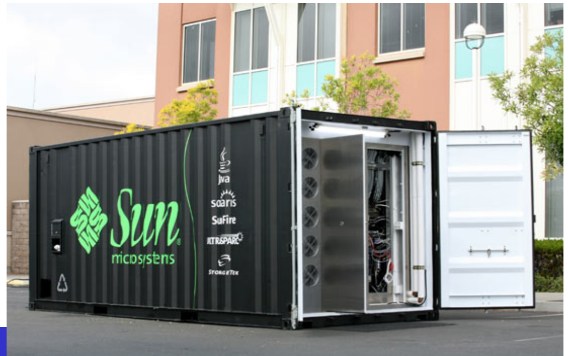
Container-based Data Center
